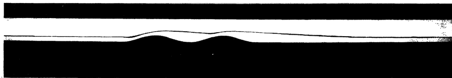
Figure 1. A photograph indicating the free-surface profile for flow at a Reynolds number of approximately 12. The flow is from right to left. The free surface of the liquid in the central portion of the channel is indicated by the lower edge of the thin line which derives from the meniscus on the side wall of the channel; the slight thickening of this line on the leeward side of the humps indicates the presence of some local structure near the side walls of the channel. The distance between the crests of the two humps in the channel bed is 100 mm.
